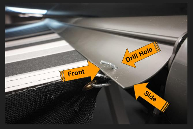
Drill 1/4 inch hole 1 3/4 inches from side x 1/2 inch from front
