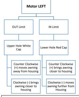
All negative (-) adjustments will only be noticed when the awning is under motion and comes to a stop. At that time, the awning will respond to positive (+) adjustments either towards the housing during IN limit or away from housing during OUT limit. **MOTOR MUST BE MOVING WHEN SETTING NEGATIVE (-) LIMITS**
