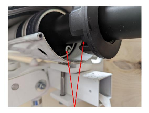
**Step 10**—Insert new motor into the tube. Be sure to line up the motor drive, motor crown and motor crown collar to the corresponding grooves
