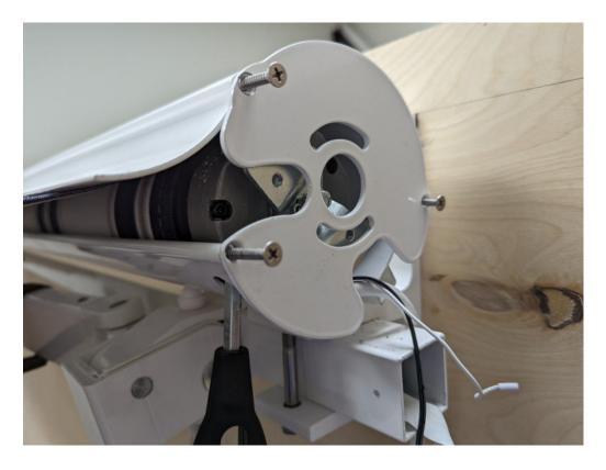
**Step 6**—Remove the 3 screws at the end of the plate
