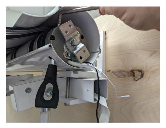
**Step 8**—Using a 90° #2 Phillips head screw driver, hold the screw and use the manual override to unscrew the retention screw. You will have to turn the override in and out so that too mush fabric isn't built up. Pull override handle down and out once the screw has been removed.
